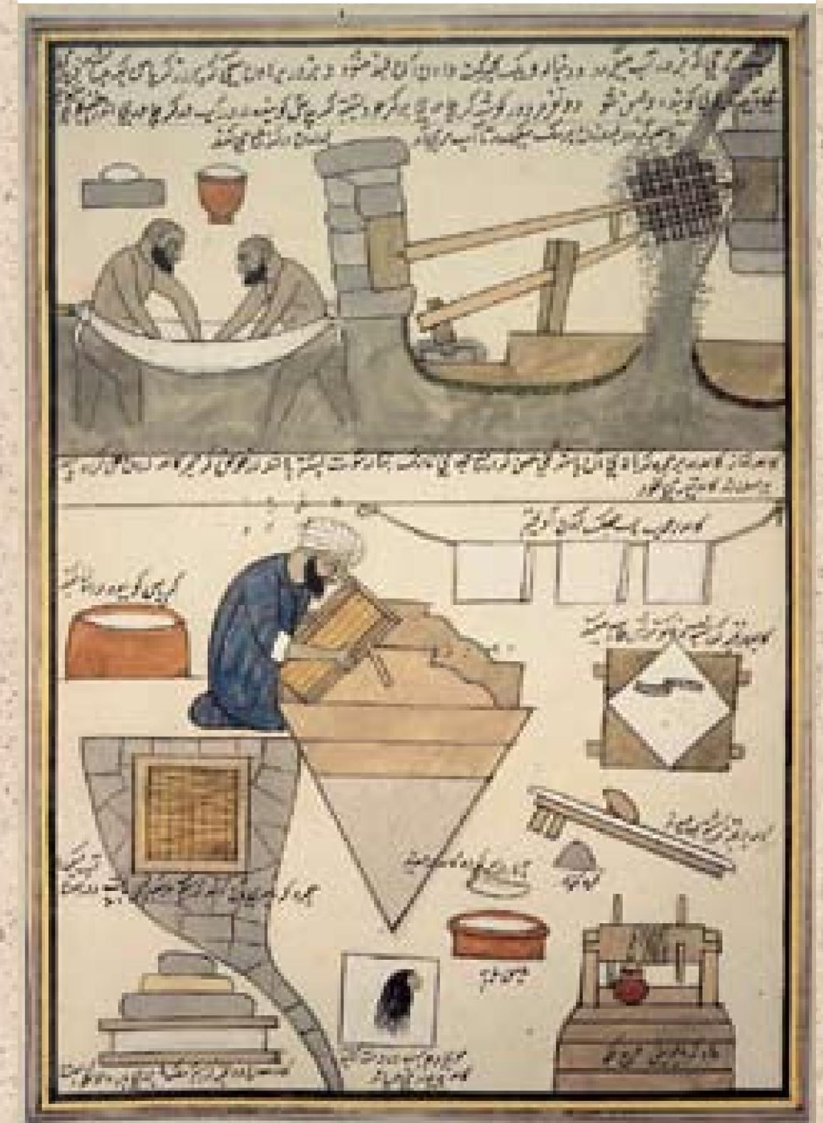
Papermaking methods are pictured in a Kashmiri trades manuscript from the mid-1800s. In the upper left a water-powered wooden stomper is depicted. Motion on the grid-wheel end produced by the water acts to force the trip-hammer up and down to pound a pile of cloth into pulp.
